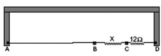
connected to it) are also available Connections are to be made to measure the unknown resistance X using the principle of Wheatstone bridge. Answer the following questions.
