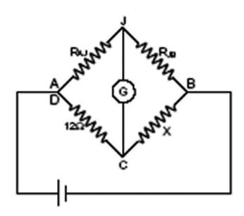
$$\frac{R_{AB}}{R_{AB}} = \frac{0.6 \,\rho}{0.4 \,\rho} = \frac{12 \,\Omega}{X} \Rightarrow X = 8 \,\Omega$$
